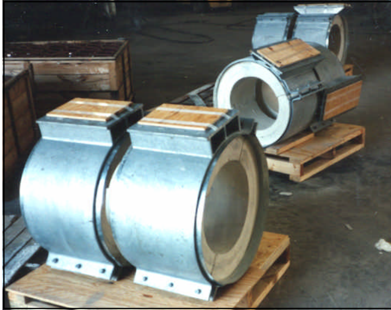
24" Sliding Hotshoes with FireTemp® Material
