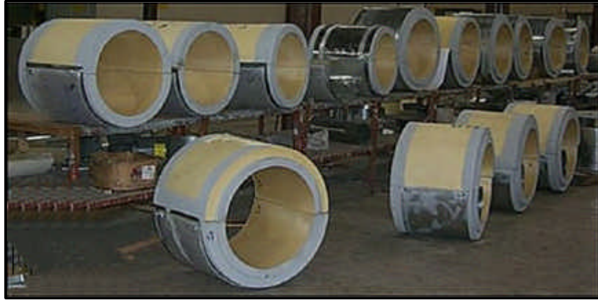
Cold Supports being assembled for shipment
